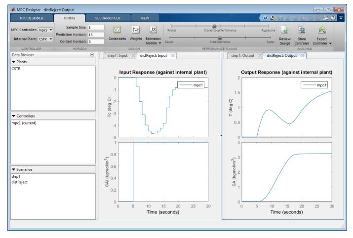
In the **Output Response** plots, once the reactor concentration, **CA**, approaches 3 kgmol/m³, the reactor temperature, **T**, starts to increase. Since there is only one manipulated variable, the controller makes a compromise between the two competing control objectives: Temperature control and constraint satisfaction. A softer output constraint enables the controller to sacrifice the constraint requirement more to achieve improved temperature tracking.
