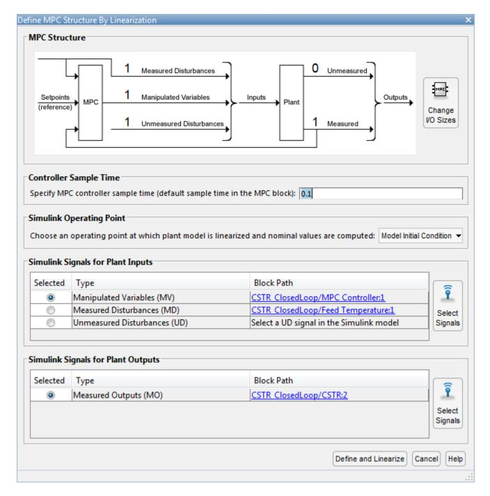
The manipulated variable, measured disturbance, and measured output are already assigned to their respective Simulink signal lines, which are connected to the MPC Controller block.
