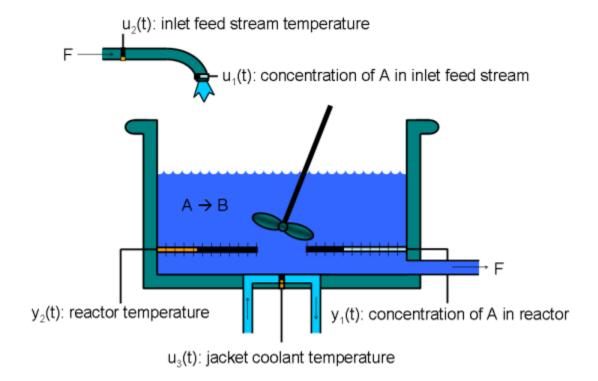
An inlet stream of reagent A feeds into the tank at a constant rate. A first-order, irreversible, exothermic reaction takes place to produce the product stream, which exits the reactor at the same rate as the input stream.
