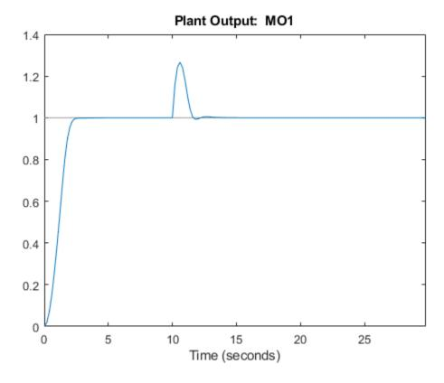
MV constraint has been slightly violated while MO constraint has been violated more. Penalize more output constraint and rerun the simulation.
