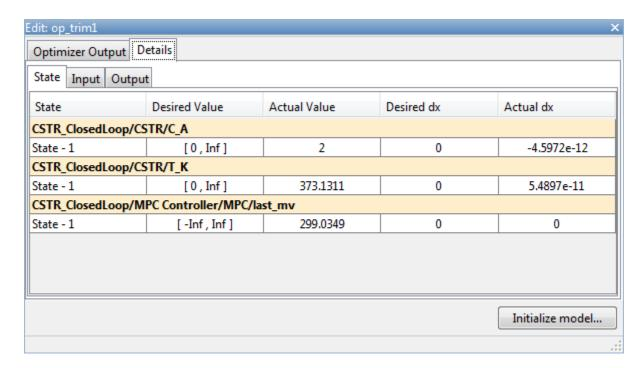
In the Edit dialog box, on the **State** tab, in the **Actual dx** column, the near-zero derivative values indicate that the computed operating point is at steady-state.
