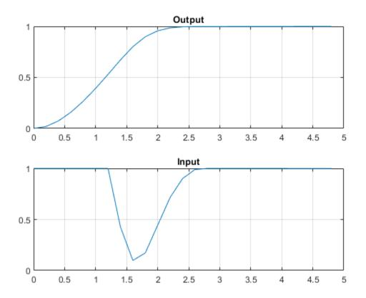
If at any time during the simulation you want to check the optimal predicted trajectories, it can be returned by mpcmove as well. Assume you want to start from the current state and have a set-point change to 0.5, and assume the measured disturbance is gone.
