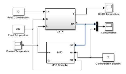
The CA signal can now be used to define output specifications for calculating a model steady-state operating point.
