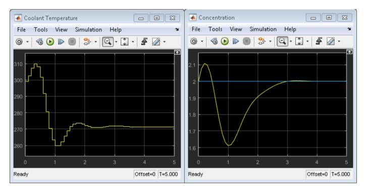
The **Concentration** output response is similar to the **UD\_reject** response, however the settling time is around 1 second later. The different result is due to the mismatch between the linear plant used in the **MPC Designer** simulation and the nonlinear plant in the Simulink model.
