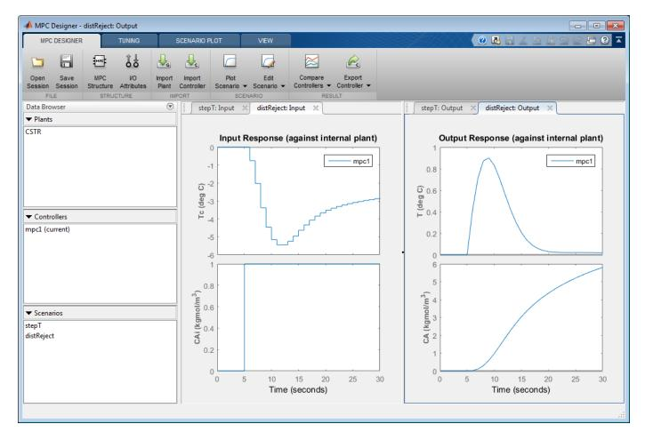
In the **Output Response** plots, the controller returns the reactor temperature,  $\mathbf{T}$ , to a value near its setpoint as expected. However, the required control actions cause an increase in the output concentration,  $\mathbf{CA}$  to 6 kgmol/m<sup>3</sup>.
