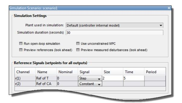
The default scenario is configured to simulate a step change of 2 degrees in the reactor temperature, T, at a time of 5 seconds.
