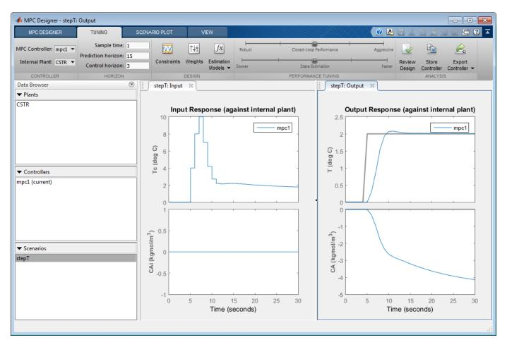
The **Input Response** plot shows the constrained manipulated variable control actions. Even with the constrained rate of change, the coolant temperature rises quickly to its maximum limit within three control intervals.
