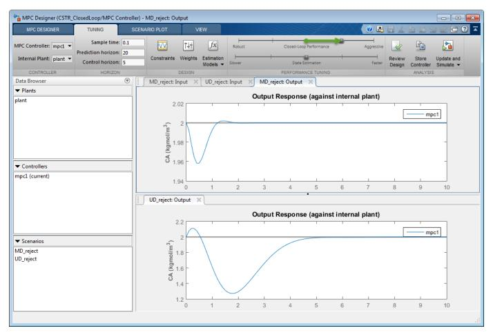
Drag the **State Estimation** slider to the right, which leads to more aggressive unmeasured disturbance rejection. Drag the slider until the **UD\_reject: Output** response reaches steady state in less than 3 seconds.
