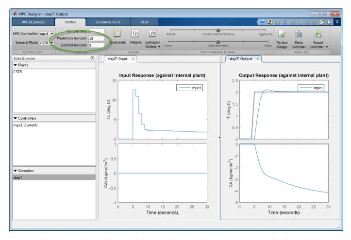
The response plots update to reflect the new horizons. The **Input Response** plot shows that the control actions for the manipulated variable violate the required coolant temperature constraints.
