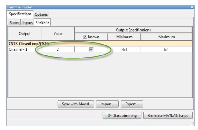
In the Trim the model dialog box, in the **Outputs** tab, check the box in the **Known** column for Channel - 1 and specify a **Value** of 2.
