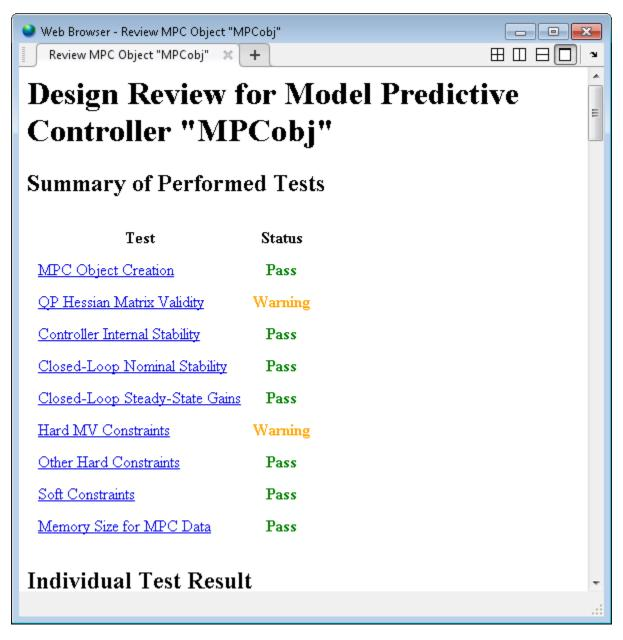
In this example, the review command found two potential issues with the design. The first warning asks whether the user intends to have a weight of zero on the C\_A output. The second warning advises the user to avoid having hard constraints on both MV and MVRate.
