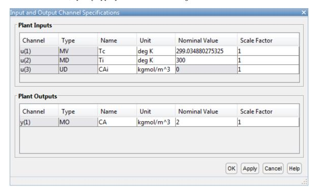
The **Nominal Value** for each signal is the corresponding steady-state value at the computed operating point.
